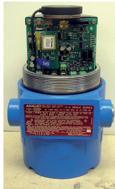
Integrated electronics and communications in a class 1 div 1 enclosure, together with a suite of x-proof sensors provide for an easy to install, robust, reliable and certified solution to track and monitor HAZMATs.
