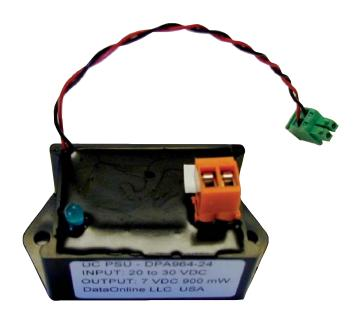
This miniature power supply module fits on the internal chassis plate inside the DPW range of WRTU's and replaces the Solar Panel as the prime battery charging power source. It is only for use with 7.4 Volt rechargeable Lithium-ion batteries.
