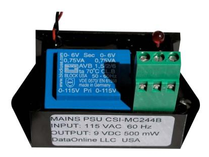
This miniature power supply module fits on the internal chassis plate inside the DPW800 range of WRTU's and replaces the Solar Panel as the prime battery charging power source.
