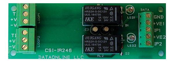
This two channel RELAY ISOLATION board is used in conjunction with the range of DPW Dataport WRTU's and isolates the analog inputs from each other. Note that each time an analog channel is sampled, the Dataport is electrically connected to that specific input.
