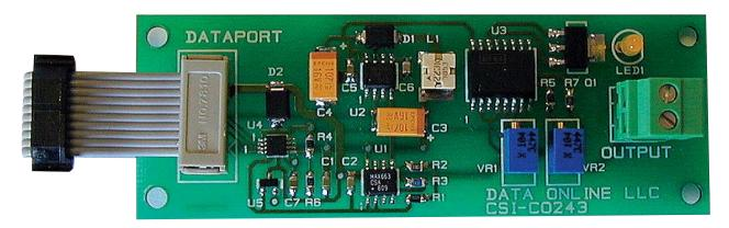
This small printed circuit board fits on to the 4 fixing pillars on the DPW series controller boards and connects into the "ALARM" connector on these boards.
