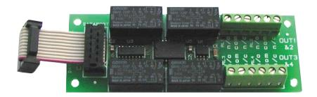
This small printed circuit board fits on to the 4 fixing pillars on the DPW series controller boards and connects into the "ALARM" connector on these boards.
