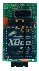
This small module "plugs on" to the main pcb of the DPW844 WRTU and allows the Dataport to communicate at 2.4 GHz with up to 4 DPR4xx Remote Sensor units. The module has its own onboard antenna and does not normally need an external antenna for correct operation. The 4 Remotes can each be up to 1000 feet away from the DPW444 WRTU under ideal conditions.
