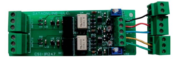
This two channel GALVANIC ISOLATION board is used in conjunction with the range of DPW800 Dataport WRTU's and isolates the external analog inputs from each other and the host Dataport. Since the WRTU printed circuit board needs to be modified to use this module, this is NOT suitable for field upgrades.
