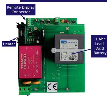
This power supply module fits inside the DPW range of WRTU's and replaces the Solar Panel and the 2.5 AHr rechargeable lead-acid battery. It also supports the use of the DPA930 remote displays without any further equipment.
