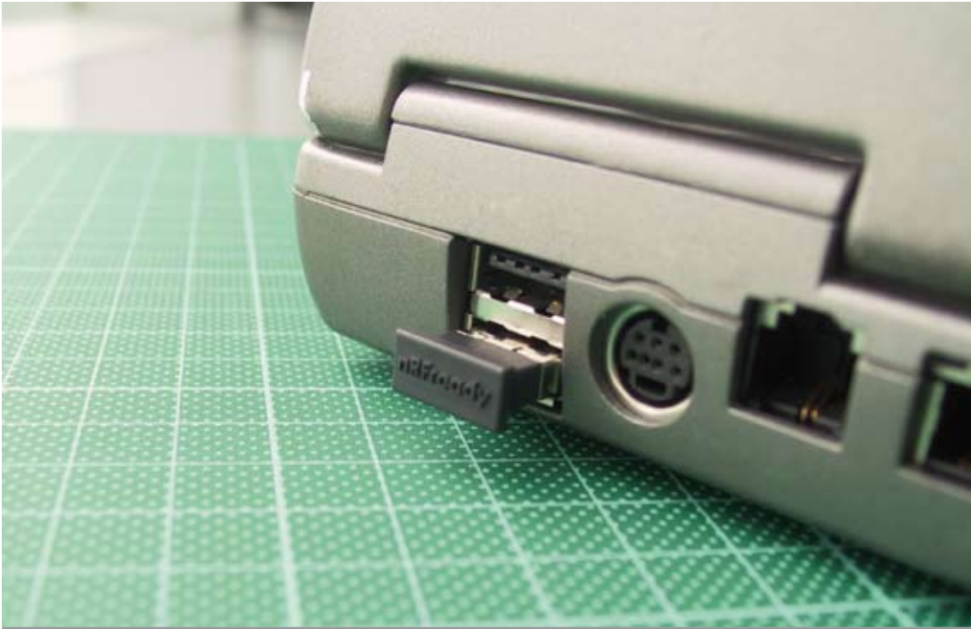
Figure 2: The nRF24LU1+ allows PC peripheral manufacturers to make tiny USB dongles with a physical profile that hardly extends beyond the USB port of the host computer
