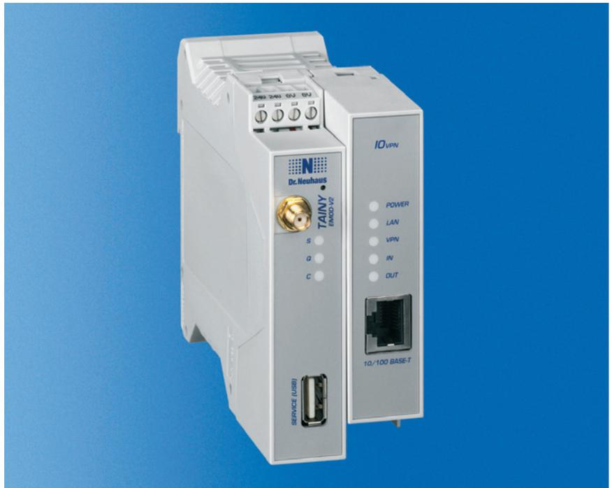
The TAINY EMOD-V2-IO from Dr. Neuhaus Telekommunikation combines a GPRS/EDGE\* wireless modem, a VPN (Virtual Private Network) router and a firewall in a single device. As a result, it is possible to transport highly sensitive data wirelessly and securely via the GSM network.
