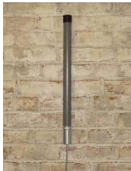
SignalFire Gateway In a Stick™ Integrated antenna and Gateway
