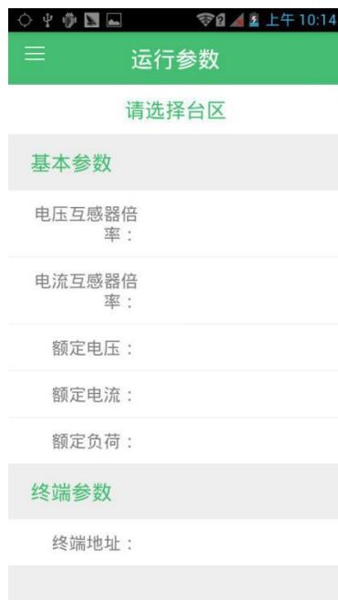
By sliding to the left and select monitored area, the relevant operating parameters of monitored area will show on the page.
