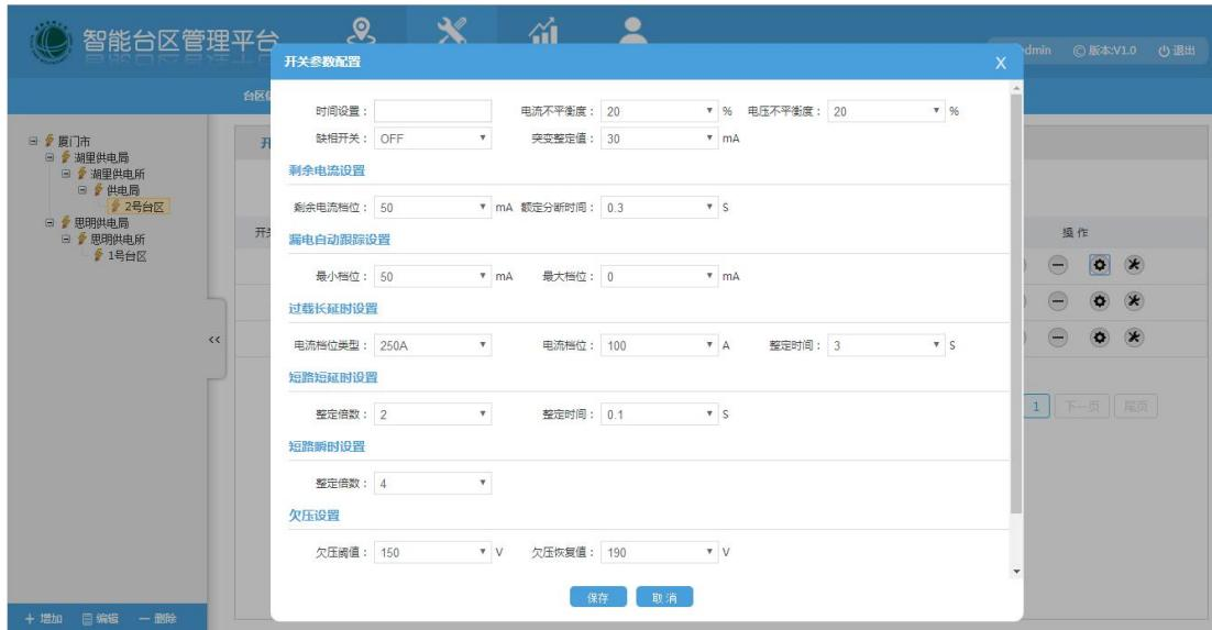
◆ **Terminal switch parameters:** click on the “Set” button in the protection switch list to load the real-time terminal switch parameters, as shown below:
