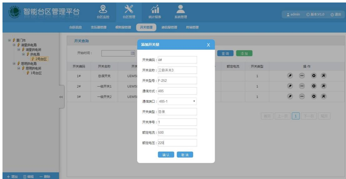
◆ **To edit protection switch:** select the protection switch information click the “Edit” button and protection switch form pop up, then fill in the relevant information and save,as shown below:
